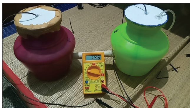
Figure 1: Simple construction of double microbial fuel cell chamber.
