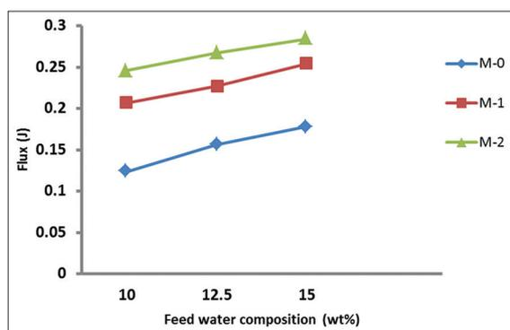
**Figure 5:** Flux versus wt.% of water in feed mixture for pristine hydroxy propyl cellulose/poly (vinyl pyrrolidone) (HPC/PVP) blend membrane (M0) and mixed matrix membranes of HPC/PVP-1(M1), HPC/PVP (M2).
