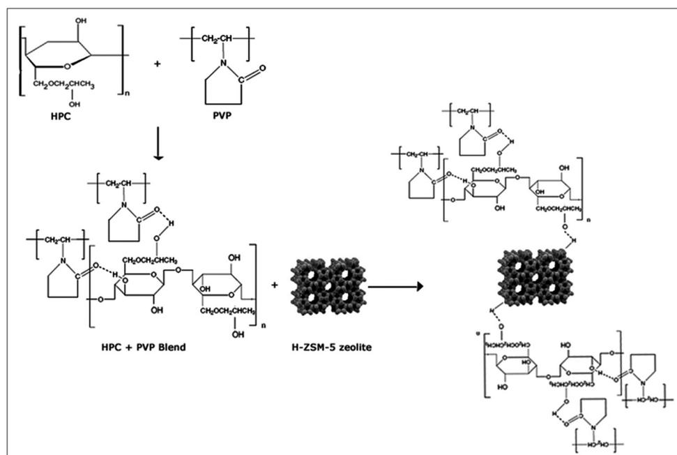
**Scheme 1:** Schematic representation of the interaction between H-ZSM-5 and hydroxy propyl cellulose/poly(vinyl pyrrolidone) blend membrane.
