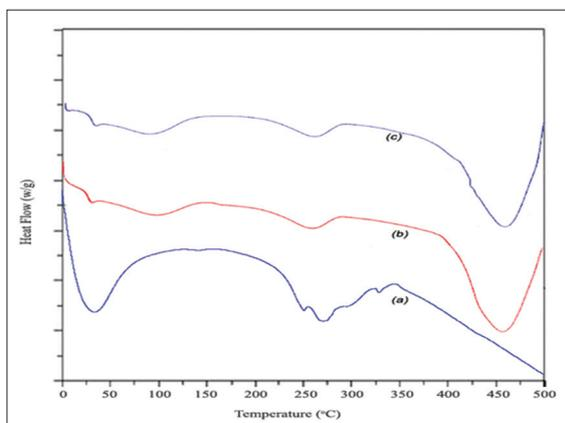
**Figure 2:** Differential scanning calorimetry thermograms of unfilled hydroxy propyl cellulose/poly (vinyl pyrrolidone) blend membrane (a), and H-ZSM-5 loaded membranes with 5 wt.% (b), and 10 wt.% (c).
