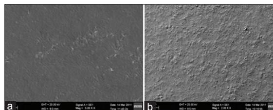
**Figure 3:** Surface scanning electron micrograph images of unfilled hydroxy propyl cellulose-poly (vinyl pyrrolidone) blend membrane (M0) (a), and H-ZSM-5 filled membrane (M1) (b).
