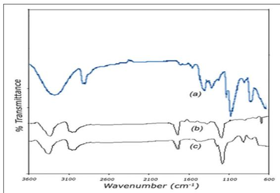
**Figure 1:** Fourier transform infrared spectroscopy spectra of (a) Pure H-ZSM-5, (b) M0, (c) M1 membranes.
