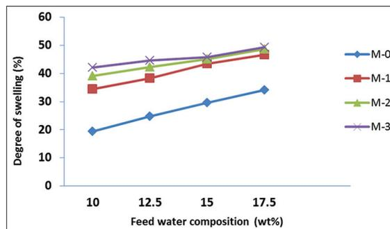
**Figure 4:** Degree of swelling of pristine hydroxy propyl cellulose/poly (vinyl pyrrolidone) blend membrane (M0) and mixed matrix membranes of HPC/PVP blend membranes (M1, M2 and M3).
