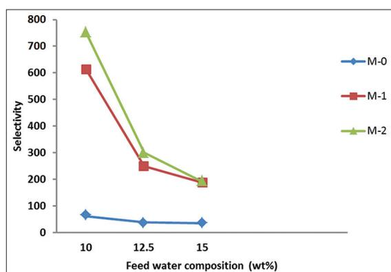
**Figure 6:** Selectivity versus wt.% of water in feed mixture for pristine hydroxy propyl cellulose/Poly (vinyl pyrrolidone) (HPC/PVP) blend membrane and mixed matrix membranes of HPC/PVP-1(M1), HPC/PVP (M2).
