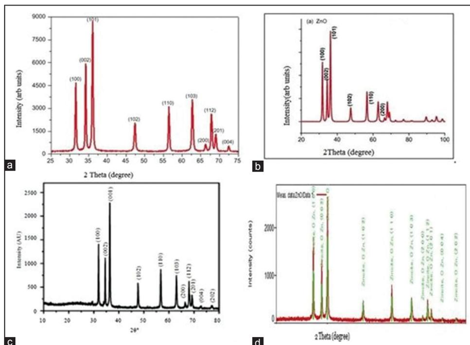
**Figure 2:** Powder X-ray diffraction (a) with glycine as fuel, (b) with citric acid as fuel, (c) with urea as fuel, and (d) with raphanus sativus as fuel.
