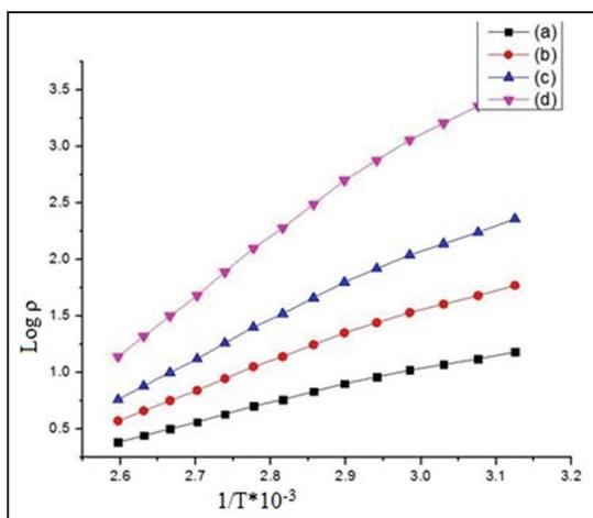
**Figure 4:** DC conductivity studies of zinc oxide nanoparticles (a) with glycine as fuel, (b) with citric acid as fuel, (c) with urea as fuel, and (d) with raphanus sativus as fuel.
