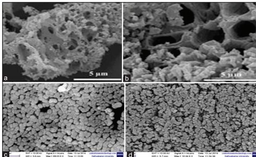
**Figure 3:** Field emission scanning electron microscopy images of zinc oxide nanoparticles (a) with glycine as fuel (b) with citric acid as fuel (c) with urea as fuel and (d) with raphanus sativus as fuel.
