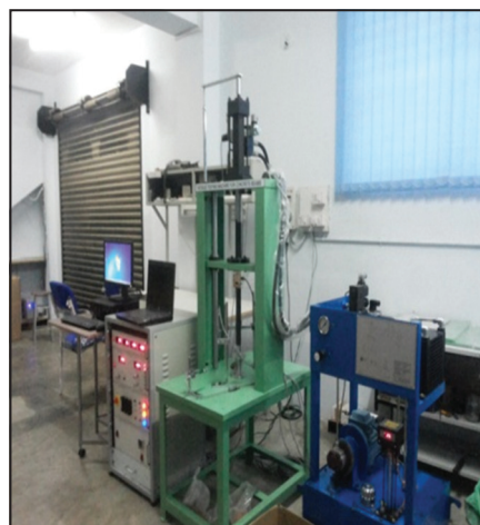
Figure 2: Apparatus for flexural fatigue testing of concrete beam.
