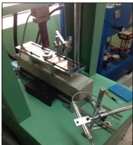
Figure 1: Test setup for fatigue testing of concrete beam specimen.
