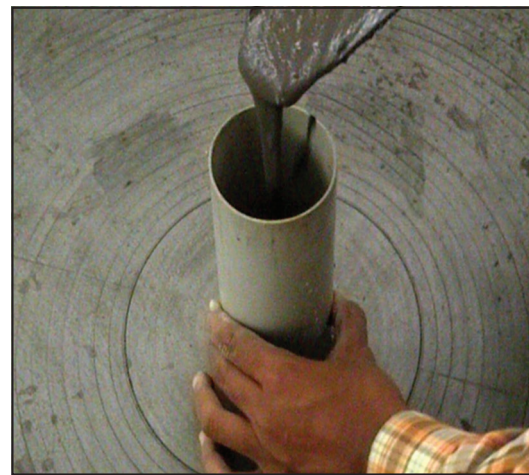
Figure 2: Placing of controlled low strength material mix into the mold.
