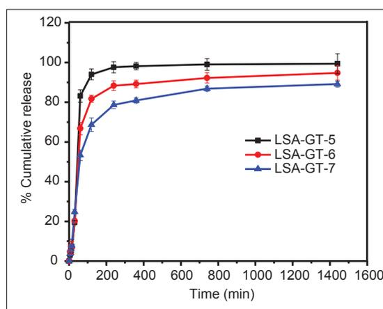
**Figure 6:** Effect of cross linker on cumulative release of pyronaridine; lignosulfonic acid/gelatin (LSA/GT) - 5 (0.4 mL), LSA/GT - 6 (0.5 mL), and LSA/GT - 7 (0.6 mL).
