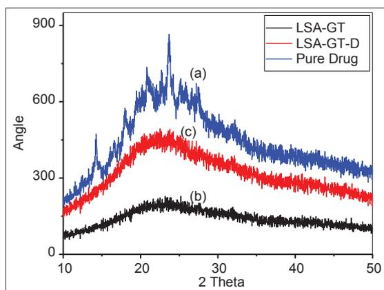
**Figure 3:** X-ray diffraction spectra of (a) Pyronaridine, (b) lignosulfonic acid/gelatin (LSA/GT) microspheres, and (c) drug-loaded LSA/GT microspheres.
