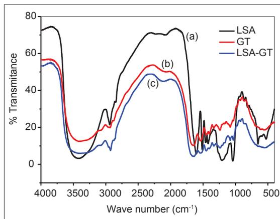
**Figure 1:** Fourier transforms-infrared spectra of (a) Lignosulfonic acid (LSA), (b) gelatin (GT), and (c) LSA/GT microspheres.
