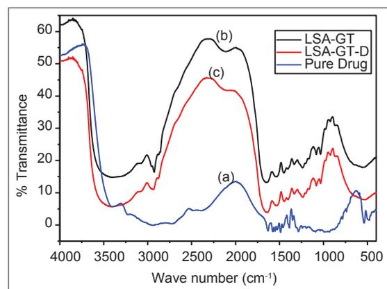
**Figure 2:** Fourier transforms-infrared spectra of (a) Pyronaridine, (b) lignosulfonic acid/gelatin (LSA/GT) microspheres, and (c) drug-loaded LSA/GT microspheres.
