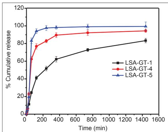
**Figure 7:** Percentage cumulative release of pyronaridine through lignosulfonic acid/gelatin (LSA/GT) microspheres containing different amounts of polymer (GT); LSA/GT - 1 (2 g), LSA/GT - 4 (3 g), LSA/GT - 5 (4 g).
