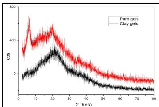
Figure .2: XRD of PAAGC hydrogels.
