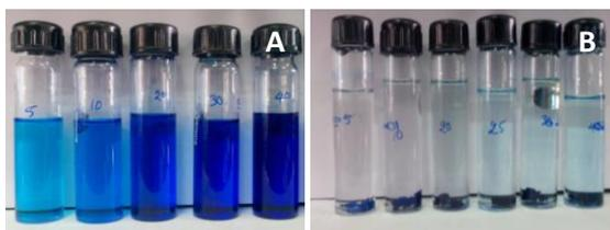
Figure 3: Optical photograph of ppm solutions of methylene blue before (A) and after (B) adsorption with PAAGC hydrogels.
