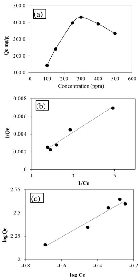
**Figure.5:**(a) Effect of concentration on equilibrium adsorption (b) lang muir isotherm (c) freundlich isotherm of PAAGC hydrogels
